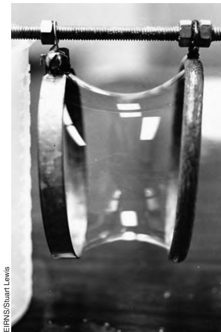
FIGURE 2. A catenoid formed by a soap film suspended between two circles.
