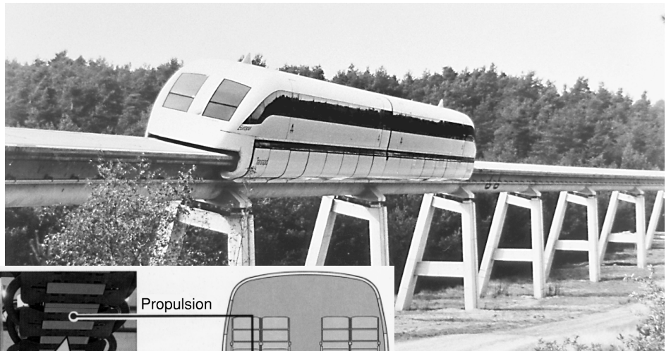
Development corridor transportation systems will incorporate magnetic levitation (maglev) technology. Above: Transrapid prototype travels at 450-500 km/hr. Left: Maglev eliminates mechanical contact between vehicle and track.
