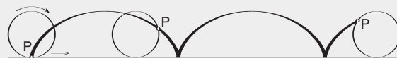
(b) The cycloid is the curve traced out by a point on a circle, as the circle rolls along a line.
